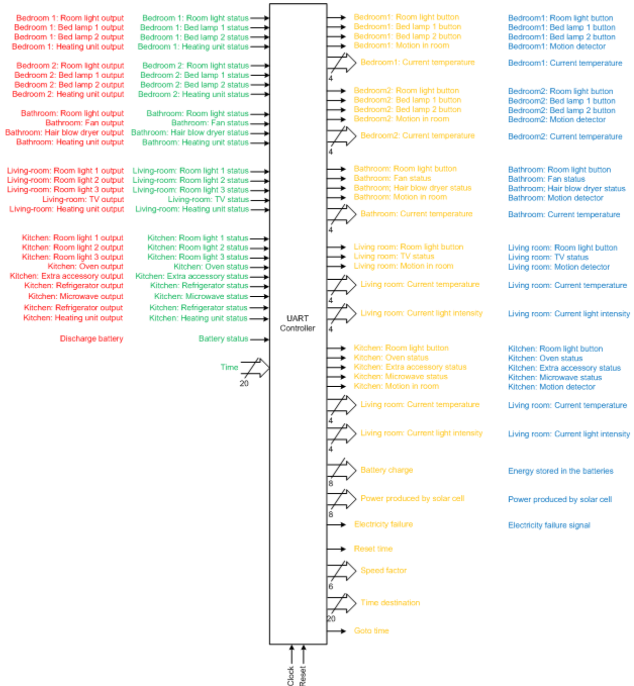
Figure 8.4.0.1: Simulator UART controller inputs and outputs
